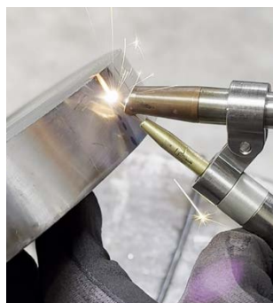
Fig. 7. Handheld laser welding for localized surface coating (left) and repair of screw flights (right)
