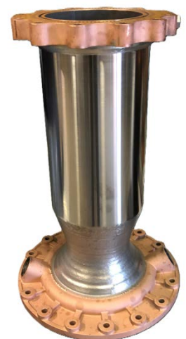
Abbildung 5: NASA – RDT Advanced Lander Propulsion Additive Cold Spray Assembly (ALPACA) [3].
