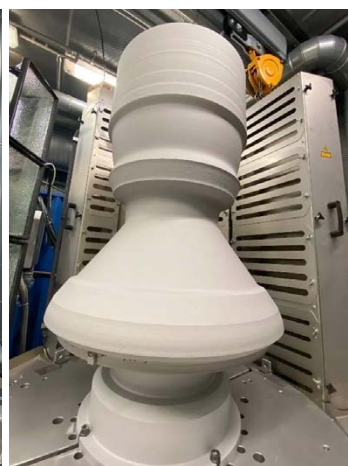
Figure 4: Cold spray of Cu-alloy – inner liner and In625 jacket on-top by ArianeGroup [2]
